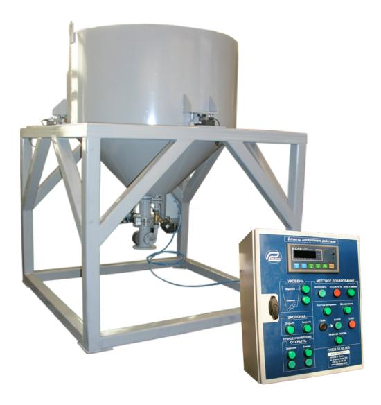
Discrete-action batcher consists of a tank, frame, cover, drain device, strain gauges, pneumatic cabinet and electrical cabinet.
